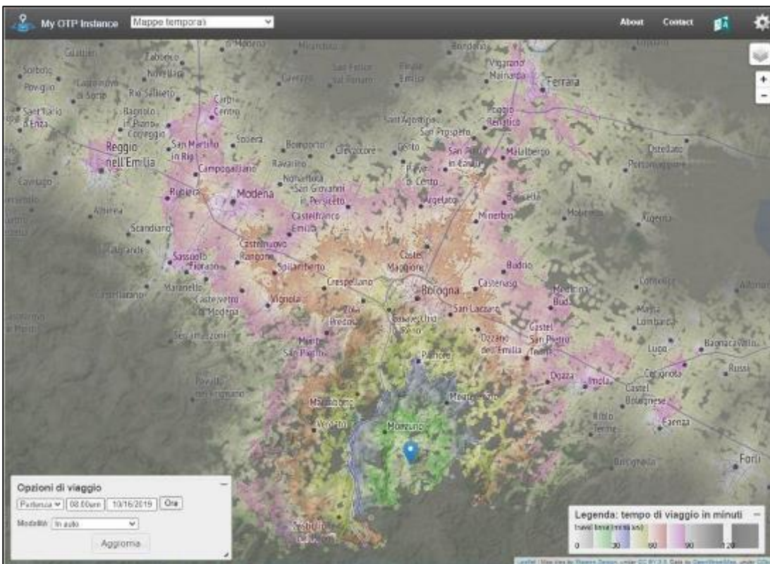
Figure 23. Example of isochrone map related to the accessibility by car of Monghidoro (reference year 2019). Elaborations using OPENTRIPPLANNER on OpenStreetmap data
